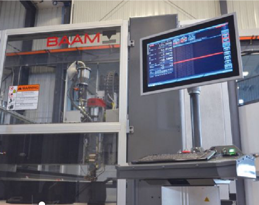
Cincinnati Incorporated's Big Area Additive Manufacturing (BAAM) system was used to produce the 3-D printed car at IMTS 2014. Courtesy: Cincinnati Inc.
