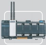
ADAM-3600-C2G Linux-based Intelligent RTU with 8x AI, 8x DI, 4x DO, and 4-slot expansion
