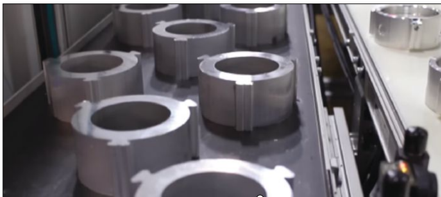
Figure 2: A camera can be placed over an inbound conveyor to take photos of each blank. Courtesy: Robotiq and Universal Robots
